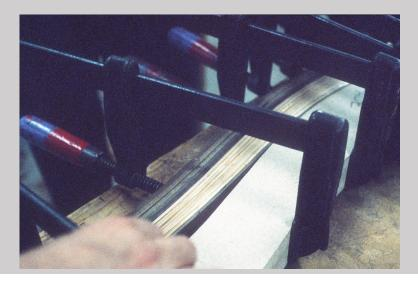
Figure 13.48i Osgood clamps the glued leg laminates between hardboard and the thick mold (photograph by Carol Ventura, 1999).
