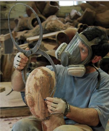
Figure 13.53d Brad Sells checks the thickness of the walls with figure 8 calipers and marks the wood with a crayon where the walls need to be thinned at his studio in Cookeville, TN (photograph by Carol Ventura, August 4, 2009).
