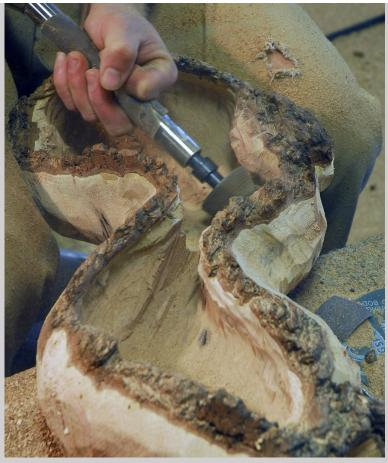
Figure 13.53b Brad Sells carves away the inner walls of the bowl with a pneumatic rotary grinder at his studio in Cookeville, TN (photograph by Carol Ventura, May 2009).
