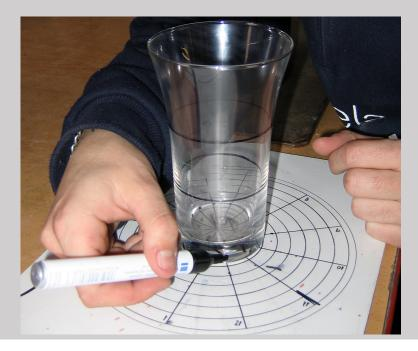
Figure 12.32d Marking glass on a template at the Glass School of the Royal Glass Factory in La Granja, Spain (photograph by Carol Ventura, 2005).
