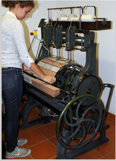
Figure 12.14d Cards are then sequentially laced together to form a continuous chain at the Lisio Foundation in Florence, Italy (photograph by Carol Ventura, 2013).
