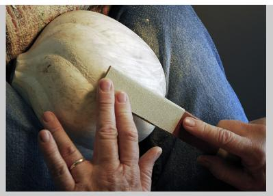
Figure 13.61m John Jordan smooths the surface with pressure sensitive adhesive sandpaper attached to a flexible piece of leather-padded walnut in Antioch, TN (photograph by Carol Ventura, 2008).
