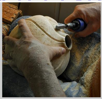
Figure 13.61k Jordan uses a pneumatic die grinder to smooth ridges in Antioch, TN (photograph by Carol Ventura, 2008).
