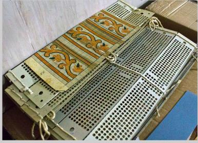
Figure 12.14a Each punched card corresponds to one horizontal row of the graphed image at the Tessitura Artigianale Giuseppe Gaggioli in Zoagli, Italy (photograph by Carol Ventura, 2013).
