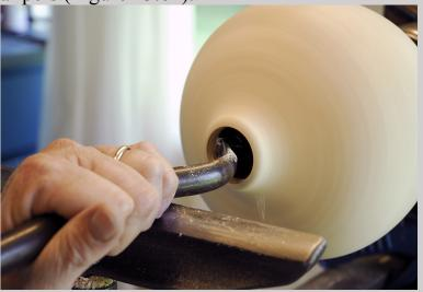
Figure 13.61e A tool rest supports Jordan's hooked tool as it bites into the inner walls of the rotating vessel in his studio in Antioch, TN (photograph by Carol Ventura, 2008).
