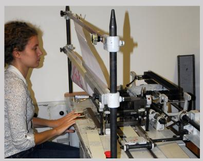
Figure 12.14c Cards being punched on a piano card puncher, following a graph paper pattern at the Lisio Foundation in Florence, Italy (photograph by Carol Ventura, 2013).
