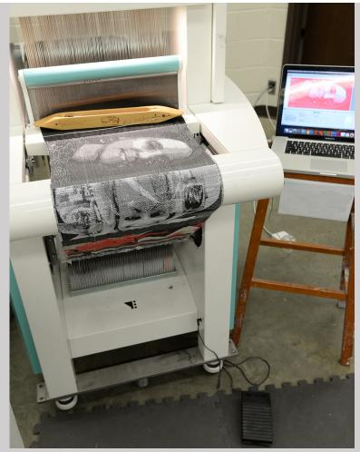
Figure 13.69a TC2 loom with woven fabric, shuttle, pedal, and laptop (photograph by Carol Ventura, 2017).
