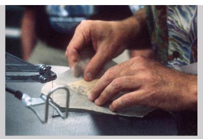
Figure 13.59a Kopf positions a tissue paper sketch over a piece of veneer so that it aligns with the grain at the Appalachian Center for Craft (photograph by Carol Ventura, 1999).
