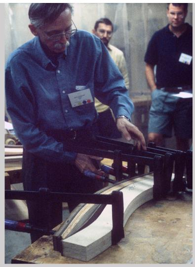
Figure 13.48h Osgood continues to clamp the glued leg laminates between hardboard and the thick mold (photograph by Carol Ventura, 1999).
