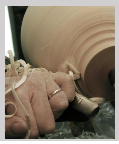
Figure 13.61d John Jordan, turns the bottom of the vessel between centers in his studio in Antioch, TN (photograph by Carol Ventura, 2008).
