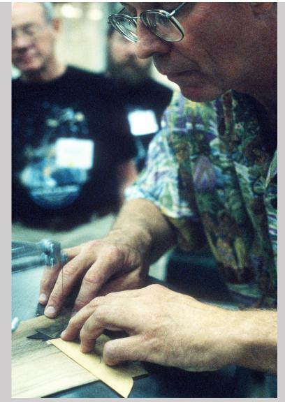
Figure 13.59d Kopf cuts veneer with a scroll saw set at a 13-degree angle to produce a double bevel cut at the Appalachian Center for Craft (photograph by Carol Ventura, 1999).
