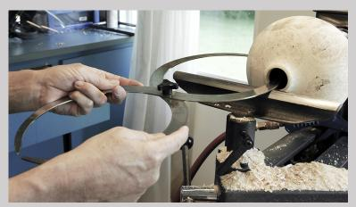
Figure 13.61f The gap between the curved ends of the figure 8 calipers shows the wall thickness in Antioch, TN (photograph by Carol Ventura, 2008).
