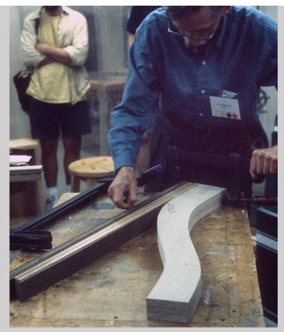
Figure 13.48g Beginning at one end, Osgood clamps the glued laminates between hardboard and the thick mold (photograph by Carol Ventura, 1999).
