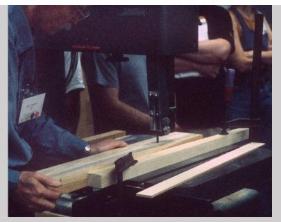
Figure 13.48b Jere Osgood cuts tapered pieces of wood on a band saw with the jig, numbering them to keep them in order for the glue-up at the Appalachian Center for Craft (photograph by Carol Ventura, 1999).
