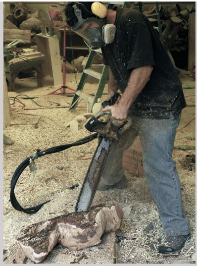
Figure 13.53a Brad Sells carves out the rough shape with a pneumatic chain saw at his studio in Cookeville, TN (photograph by Carol Ventura, September 2008).
