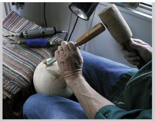
Figure 13.61h With the vessel secured between his knees and a padded table, John Jordan carves off the remains of the tenon to create a slightly concave base in Antioch, TN (photograph by Carol Ventura, 2008).
