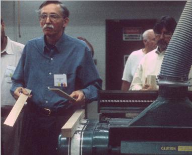
Figure 13.48d Osgood will place one of the tapered strips on the jig resting on the planer, then run them through the planer at the Appalachian Center for Craft (photograph by Carol Ventura, 1999).
