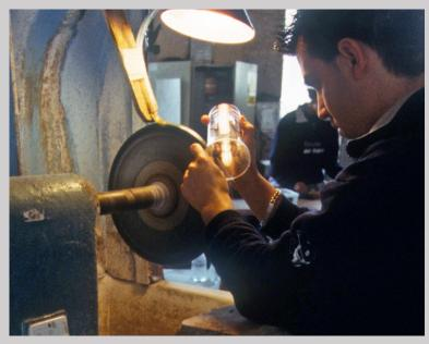
Figure 12.32f Cutting glass on a lathe at the Glass School of the Royal Glass Factory in La Granja, Spain (photograph by Carol Ventura, 2005).
