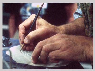
Figure 13.59b Kopf inserts a piece of carbon paper under the sketch and then traces over the lines to transfer the sketch to the veneer at the Appalachian Center for Craft (photograph by Carol Ventura, 1999).
