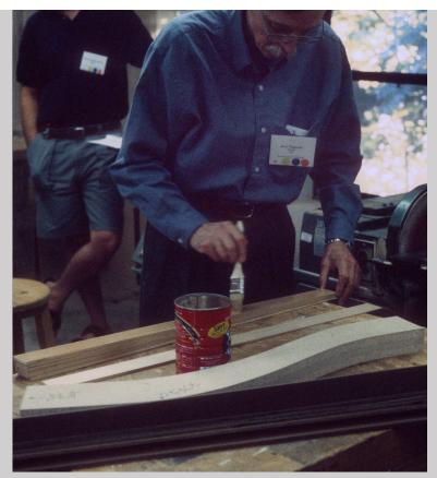
Figure 13.48f Osgood paints glue on the tapered strips of wood at the Appalachian Center for Craft (photograph by Carol Ventura, 1999).
