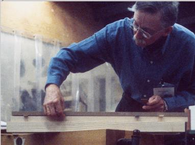
Figure 13.48a Jere Osgood inserts splines into a jig at the Appalachian Center for Craft (photograph by Carol Ventura, 1999).
