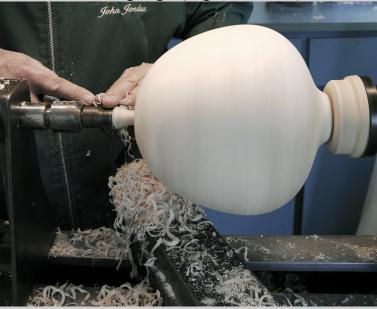
Figure 13.61g With the top of the vessel in a jam chuck and the bottom supported by the live center of the tail stock, Jordan turns away the tenon from the base in Antioch, TN (photograph by Carol Ventura, 2008).
