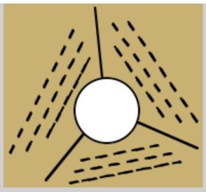
Figure 13.59c To avoid short grain problems, Kopf joins several pieces of veneer together, running the grain as illustrated (illustration by Carol Ventura).
