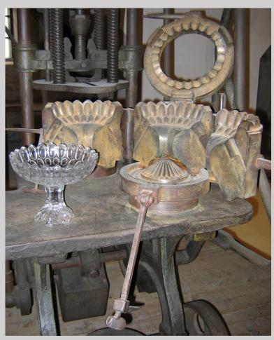
Figure 12.2c Hinged metal press mold for a pressed glass fruit bowl, Royal Glass Factory in La Granja, Spain (photograph by Carol Ventura, 2005).
