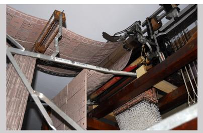
Figure 12.14e Punched cards laced together on a Jacquard head box on top of a loom with white cords that control the heddles at the Artigiana Giuseppe Gaggioli weaving studio in Zoagli, Italy (photograph by Carol Ventura, 2013).
